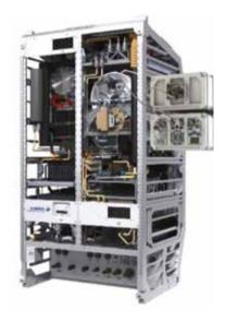
Photobioreactor integrated at LSR
