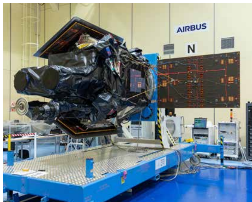
TEST FOR DEPLOYING SOLAR PANELS ©AIRBUS 2020.
